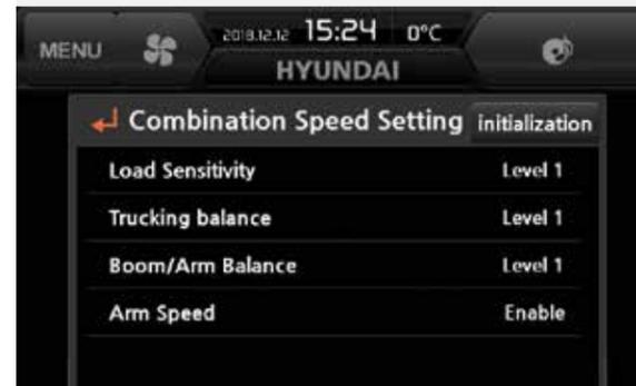
The **combination speed setting system** allows operators to balance load sensitivity and boom priority against arm and swing. Select from five levels of load sensitivity to adjust initial flow rate for boom-up and arm-in operation according to attachment weight. Ten levels of boom priority can be selected to balance boom operation against arm and swing.
