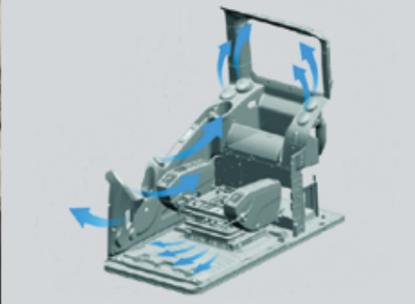
The **heating and air conditioning** system efficiently regulates and directs airflow in the cabin.
