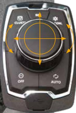
The accelerator, remote air conditioner controller and instrument cluster can be operated using the convenient jog shuttle-type **haptic controller**.
