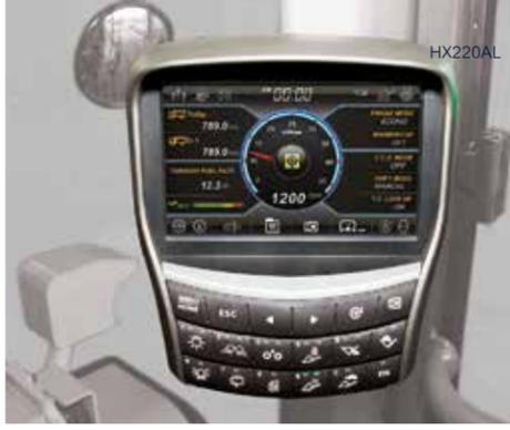
The **instrument panel** is optimised to provide quick, easy access to machine status information as you work. It features an 8-inch **touchscreen monitor** for excellent legibility.
